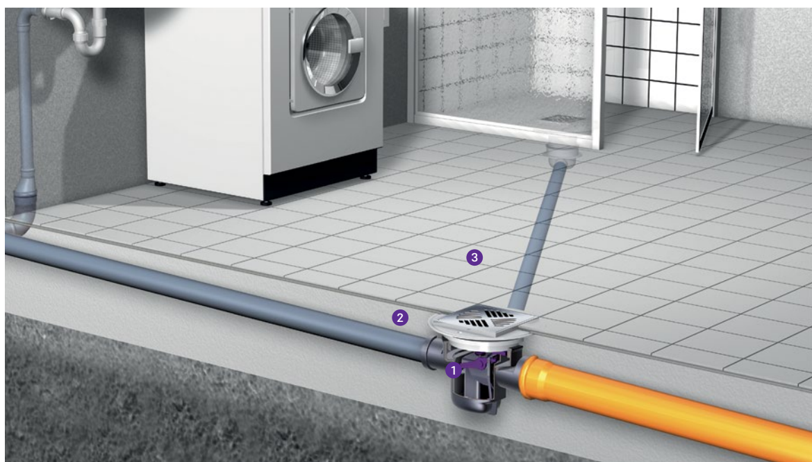
1 Drain 2 Inlet 3 Steel cover
