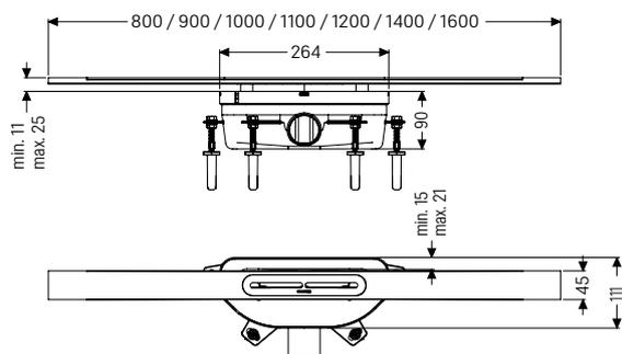
**Odour trap with 50 mm water seal**
