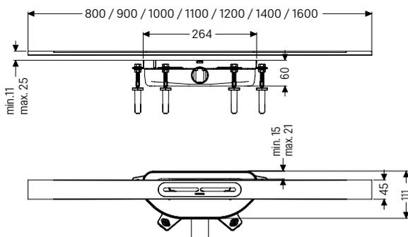
**Odour trap with 24 mm water seal**
