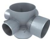
With three inlets Ø 55 mm and one outlet Ø 75 mm, with removable odour trap. The flow rate is 1.8 l/s.
