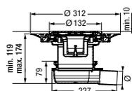
**The Ultraflat 79 without waterproofing membrane**
