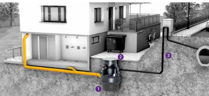
1 Pumping station 2 Engineering chamber 3 Pressure pipe
